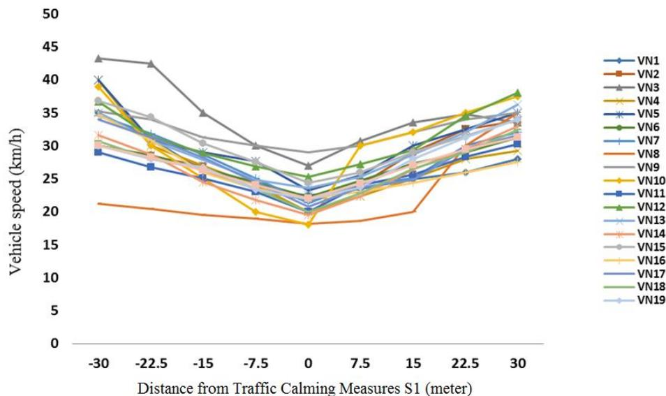
Figure 7. Speed profile of all vehicles in first TCM
