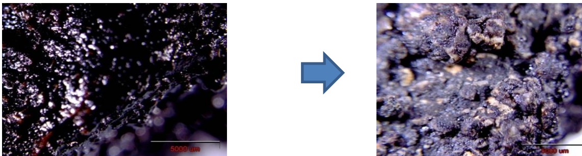
Figure 4. Micro image after boiling test with PMB with 4% Lucobit (Left: Normal, Right: Microscope image)
