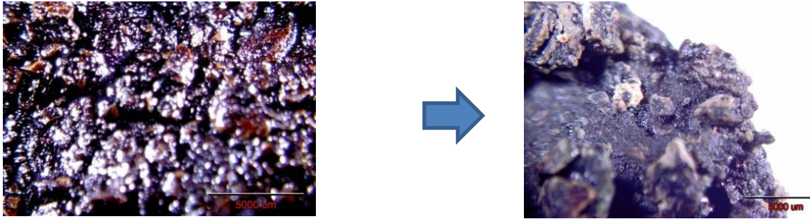
Figure 2. Micro image after boiling test with base bitumen (Left: Normal, Right: Microscope image)
