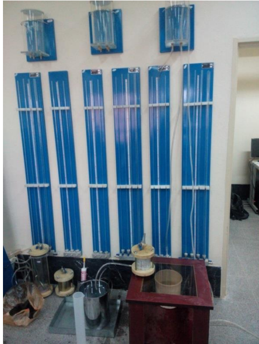
Figure 4. Permeability testing device
